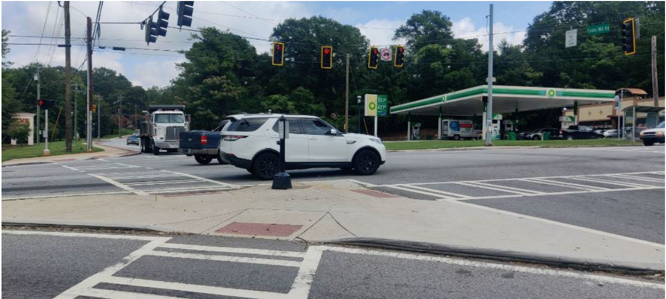
Figure 7-8: Push buttons located at the traffic island rather than at the edge of the road.
